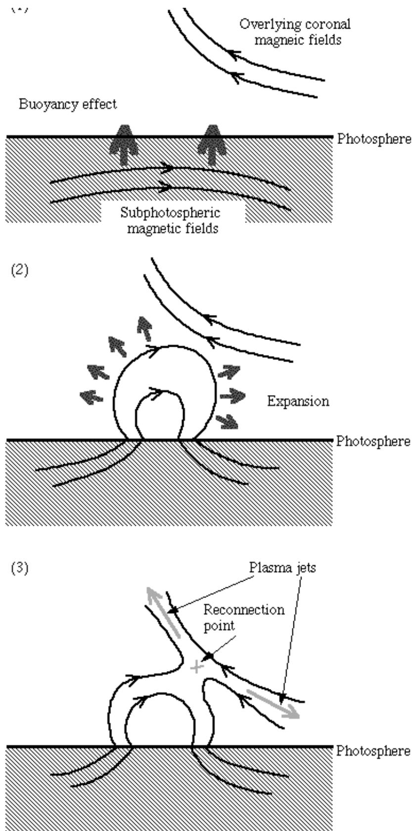
FIG.4. 1.—Schematic illustration of the emergence of the subphotospheric magnetic field from a 2-dimensional viewpoint. The subphotospheric magnetic field begins to rise because of the buoyancy effect (or Parker instability) and eventually emerges on the surface. Then, owing to the rapid decrease of the surrounding gas pressure, it begins to expand outward and finally interacts with the overlying coronal magnetic field.
