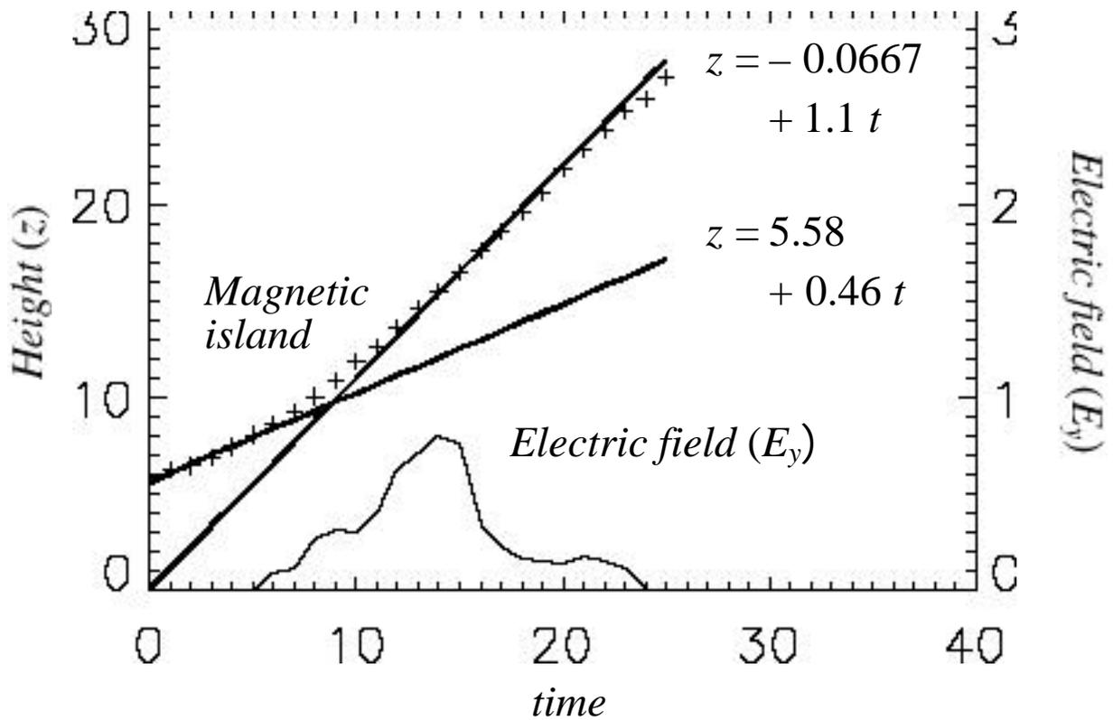
FIG. 3. 3.—Time variations of the y-component of the electric field ( $E_y$ ) at a neutral point and the height of a magnetic island of model r3, each of which are represented by a thin solid line and crosses (+), respectively. Two thick solid lines represent the result of the line-fittings applied to the time variation of the height of the magnetic island. The time ranges of such line-fittings are  $0 \leq t \leq 5$  for the first one and  $15 \leq t \leq 17$  for the second one.
