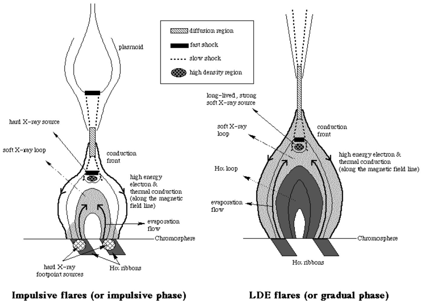
FIG. 2. 9.—Schematic illustration of a flare model based on the magnetic reconnection. For details, see the text in § 2. 5. 1.
