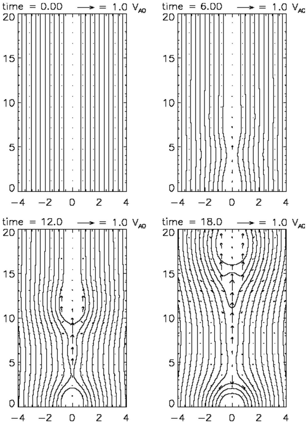
FIG. 2. 4.—Typical evolution of the present numerical simulation. Contour lines and arrows represent the magnetic field lines and velocity field, respectively. Elapsed times are  $t = 0$  (top-left),  $t = 6$  (top-right),  $t = 12$  (bottom-left), and  $t = 18$  (bottom-right), respectively. Note that part of the calculation region,  $(-4, 0) \leq (x, z) \leq (4, 20)$ , is displayed.
