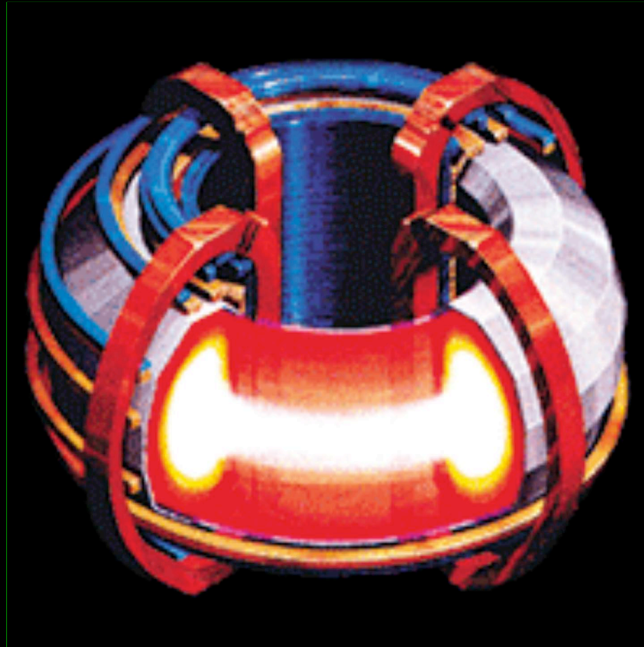
Plasma in a tokamak
