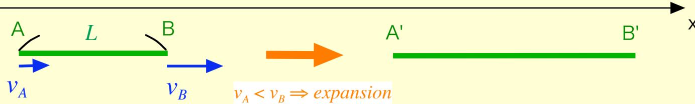
$$\text{Expansion rate} \equiv \frac{1}{L} \frac{dL}{dt} \Rightarrow \frac{1}{x_B - x_A} \frac{d}{dt} (x_B - x_A) \Big|_{x_B = x_A + \Delta x} \Rightarrow \frac{1}{\Delta x} [v_x(x_A + \Delta x) - v_x(x_A)] \xrightarrow{\Delta x \rightarrow 0} \frac{\partial v_x}{\partial x}$$
