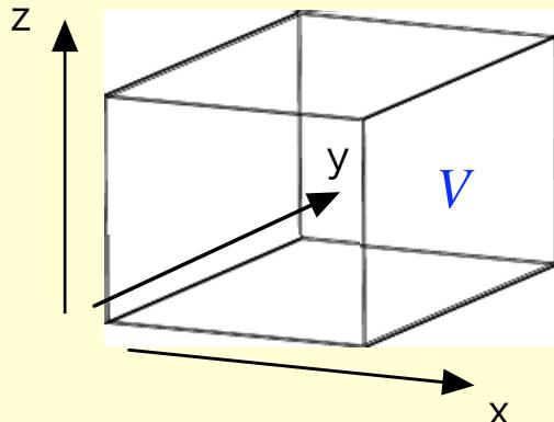
$$\text{Expansion rate} \equiv \frac{1}{V} \frac{dV}{dt} = \frac{\partial v_x}{\partial x} + \frac{\partial v_y}{\partial y} + \frac{\partial v_z}{\partial z} \equiv \nabla \cdot \mathbf{v}$$
