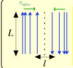
Magnetic flux is continuously supplied to diffusion region by inflow, so the magnetic flux density is almost kept constant in the region. This is different from simple diffusion (flux density decreases with time)
