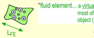
\*fluid element... a <u>virtual</u> object containing a number of particles; most of the particles keep staying inside the object (=> typical size  $L_{FE}$  >>  $l_{mfp}$ ,  $r_{G}$ )
