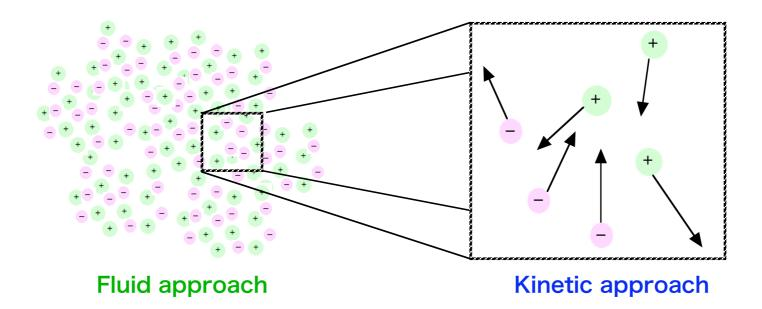
**Kinetic approach** → study microscale processes, the behavior of particles
